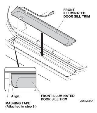
Attach the front illuminated door sill trim to the vehicle panel by removing the two adhesive backings and pressing on the trim firmly with your hands.
