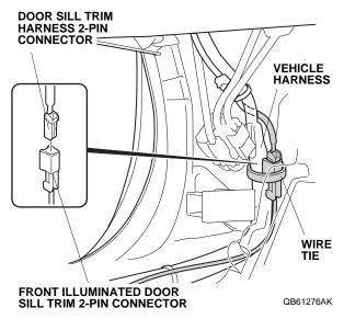
48. Using one wire tie, secure the front illuminated door sill trim 2-pin connector to the vehicle harness.
