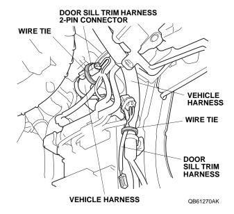
40. Plug the door sill trim harness 2-pin connector to the front illuminated door sill trim 2-pin connector.
