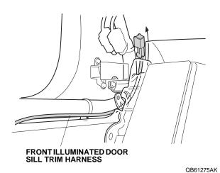
47. Plug the door sill trim harness 2-pin connector to the front illuminated door sill trim 2-pin connector.
