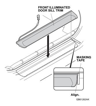
25. Using isopropyl alcohol on a shop towel, thoroughly clean the area where the protective tape will attach.
