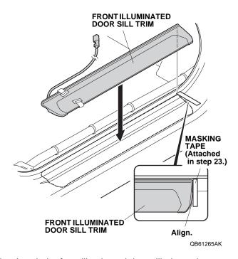
32. Attach the front illuminated door sill trim to the vehicle panel by removing the two adhesive backings and pressing on the trim firmly with your hands.
