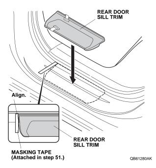
56. Attach the rear door sill trim to the vehicle panel by removing the two adhesive backings and pressing on the trim firmly with your hands.
