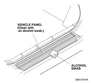
31. Position the front illuminated door sill trim with the masking tape.
